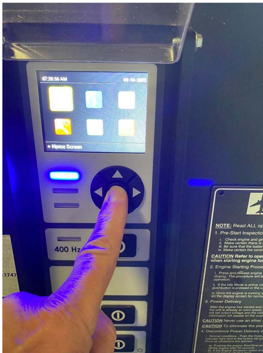
Figure 13: Press and hold the center button until the Home screen appears
