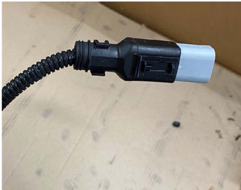
Figure 8: Electrical connector to the 4400. Both heads connect the same to the unit.
