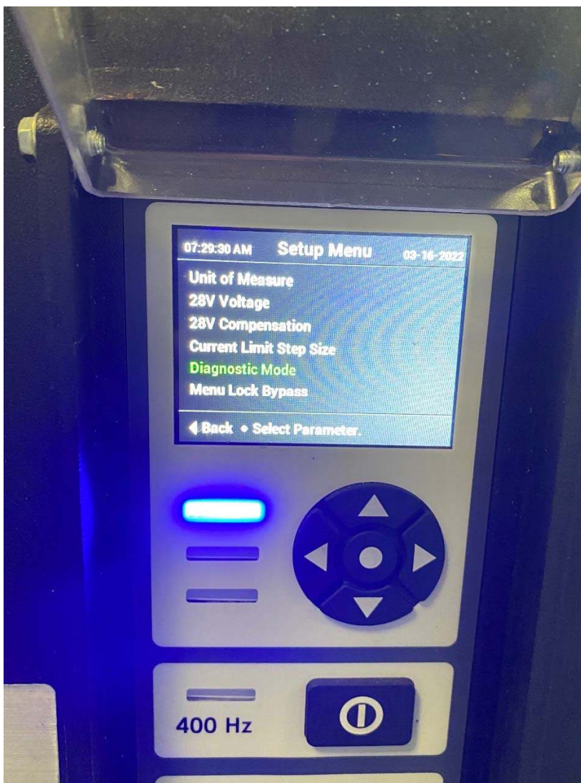
Figure 16: Use the bottom arrow to scroll until Diagnostic Mode is highlighted green
