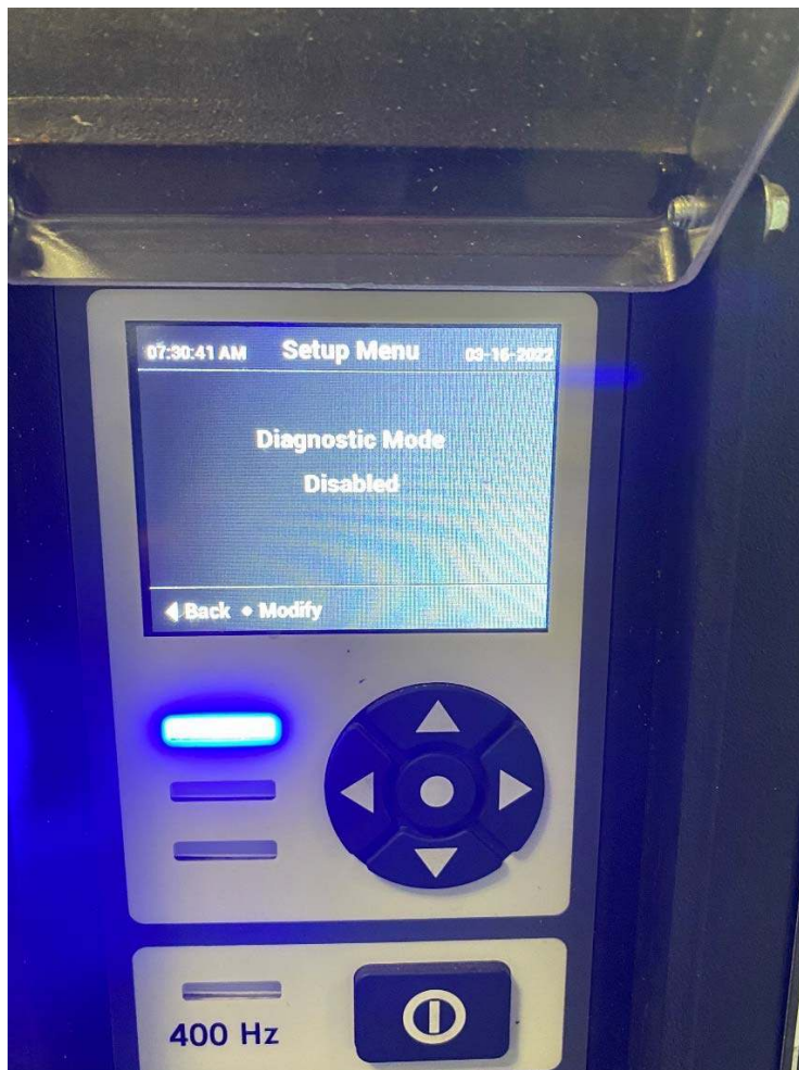
Figure 17: Press center button and Diagnostic mode will appear
