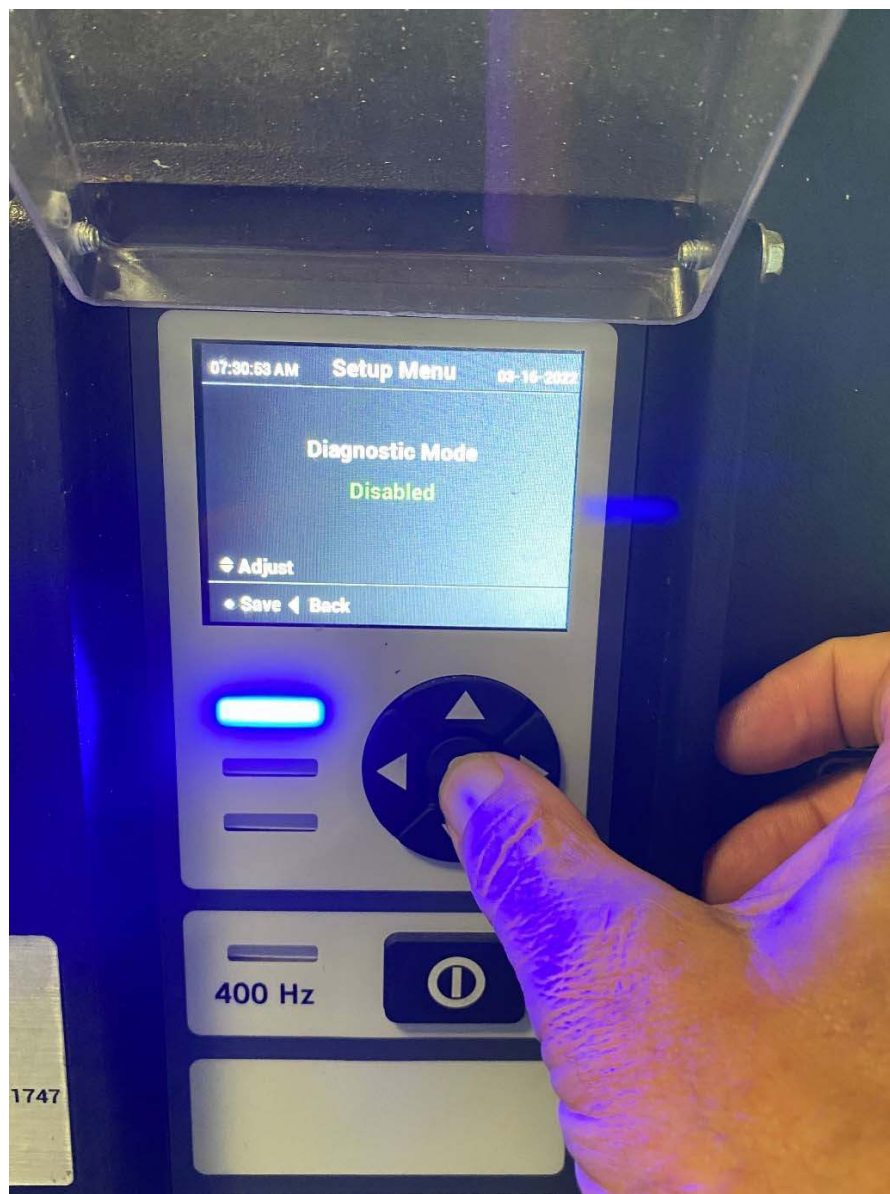
Figure 18: Press center button to highlight Disabled
