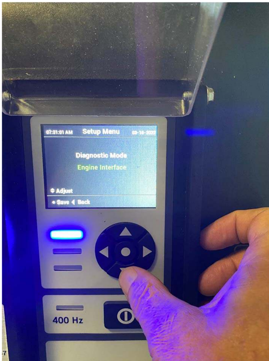
Figure 19: Use Up/Down buttons until Engine Interface is displayed and press center button to save
