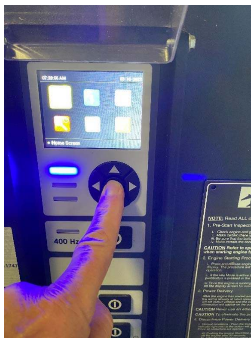
Figure 15: Press center button to enter the setup menus
