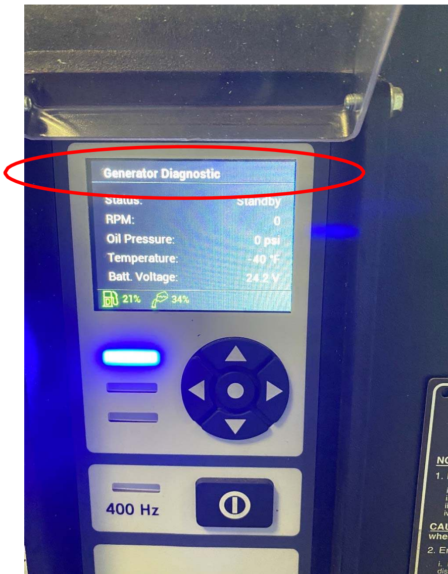
Figure 21: Note the unit is in Generator Diagnostic mode
