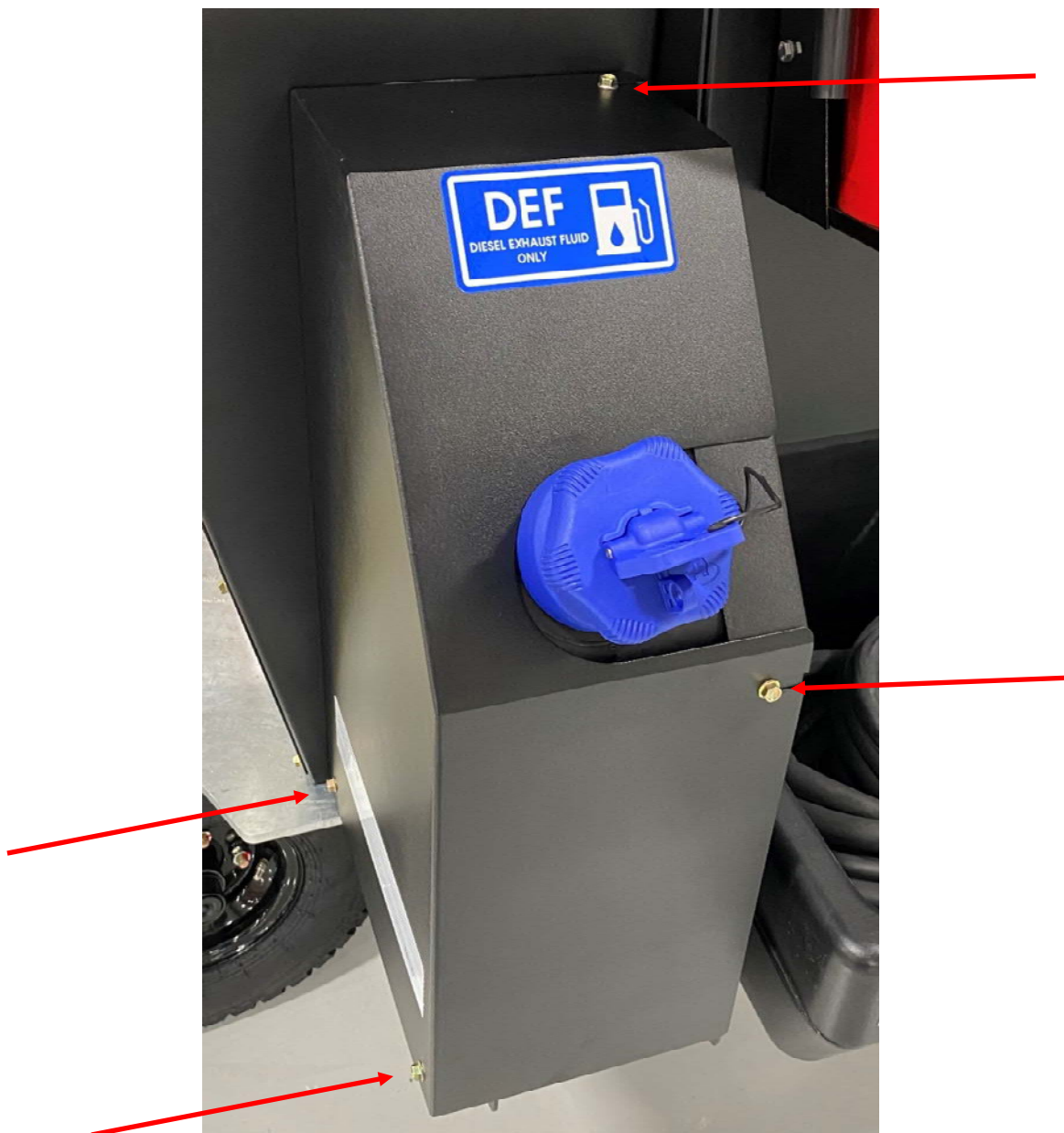
Figure 1: Remove 4 bolts per arrows.
