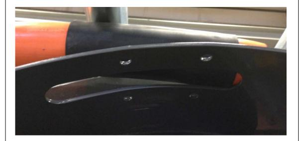
C. Fit the front cable clamp and tighten the bolts by turns, until the bolt ends are through the cable clamp.
