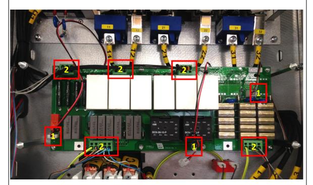
2. Disconnect / release cables from terminals marked cables that ends up having no connections.
