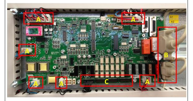
**D.** Remove the 2 x 3 wires from the MCB marked
