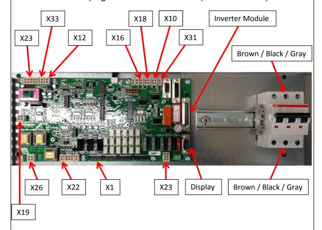
10. Check that there are no un-connected wires or plugs.
