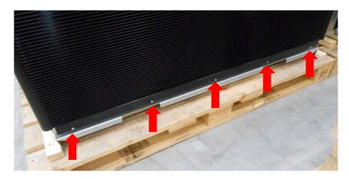
04. In the side furthest away from the compressor, drill out 4 pcs. rivets with a 5mm drill.
