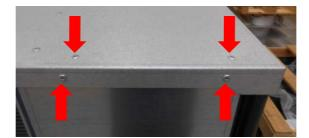
05. In the side closest to the compressor, drill out 5 pcs. rivets with a 5mm drill.
