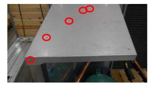
O6. Lift the module roof plate and place pieces of wood between the back plate and roof plate. Ensure that the roof plate is clear from the condenser in both sides.
