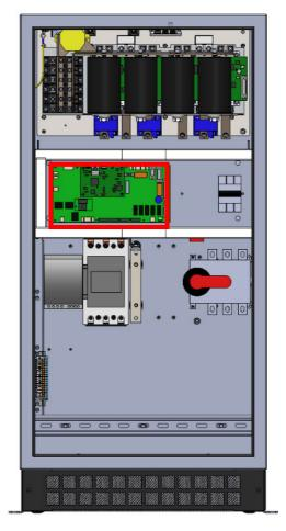
1. Remove the plug **X10** (plug No. 2 from right upper row) from the Interface Board and pull the cable out of the cable trays. (**X10** & cable removed on picture below)
