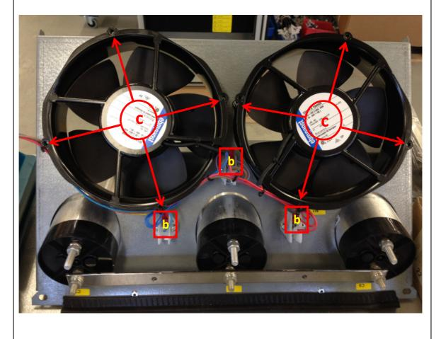
A. Retrofit the 2 fans by inserting and fasten the 2 x 4 screws. 4 Observe the fan cable position.
