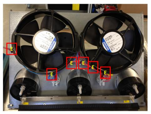
The fan/capacitor assembly is now ready to retrofit into the unit.
