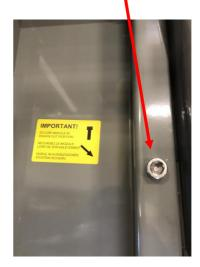
5 Disconnect the cables marked with red arrows. Retain nuts and washers for reinstallation.
