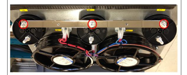
C. Connect the 2 x A-B-C-N cables and fasten the bolts / nuts (A-B-C Torque = 4 Nm / 35.4 in-lb)
