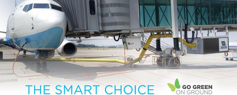
The ITW GSE 3500 provides a pleasant and welcoming atmosphere for crew and passengers as soon as they step into the aircraft. Automated Aircraft Type Detection allows the 3500 PCA to automatically adapt its airflow to the specific aircraft type - and not just an aircraft category. This not only helps to avoid operator errors - it also increases the PCA cooling performance by more than 50 % and improves the passenger comfort.
